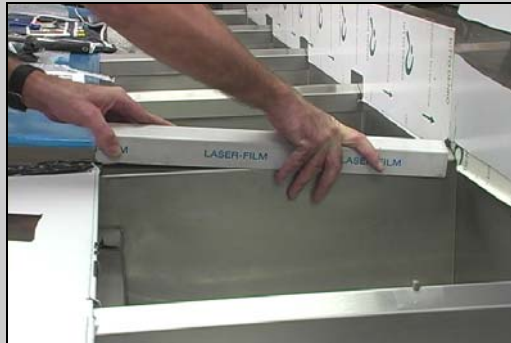
Figure 9: Place joiner strip which connects the frypots.
