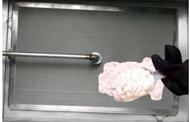
Applying filter powder to filter-leaf.
