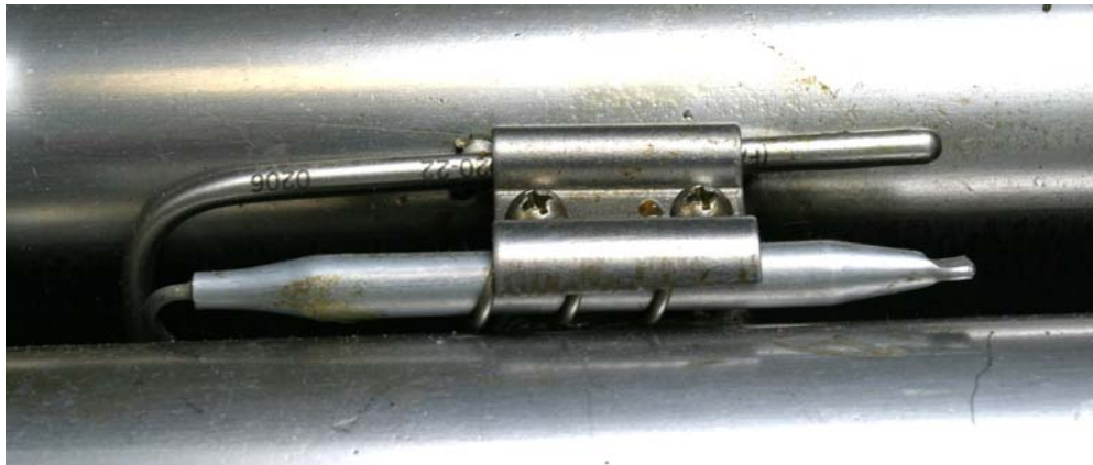
Typical high-limit/sensor probe locations and mounting hardware.
